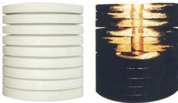
Figure 1: Clean and dirty filter insert
