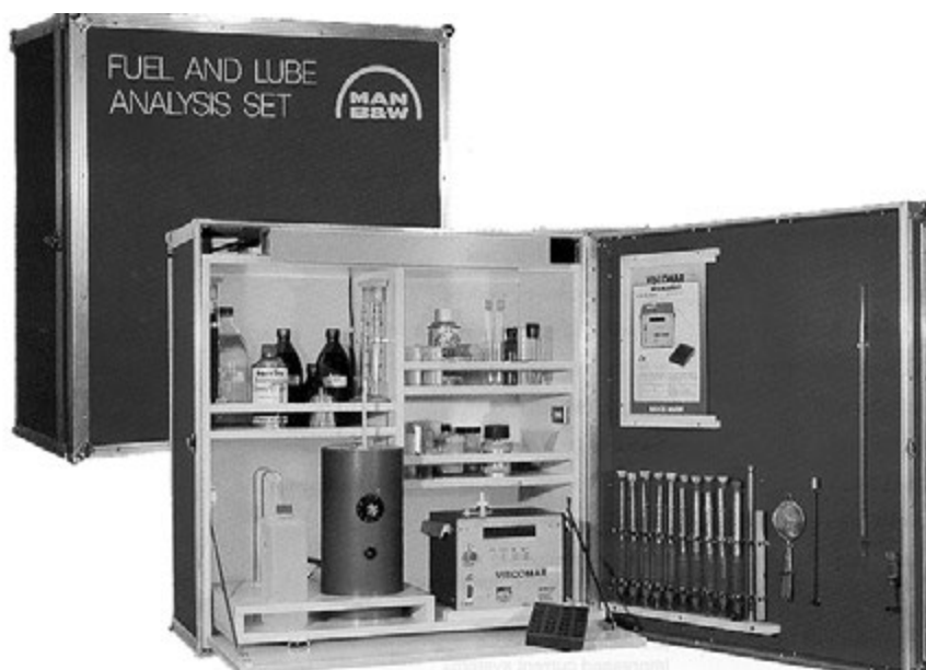
Figure 1: Test kit case A for the analysis of fuel and lubricating oil
