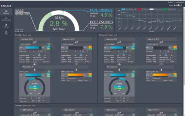
ECOLOAD advisory system providing advice on holistic powertrain operation
