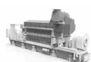
Pump on front end – common base frame
