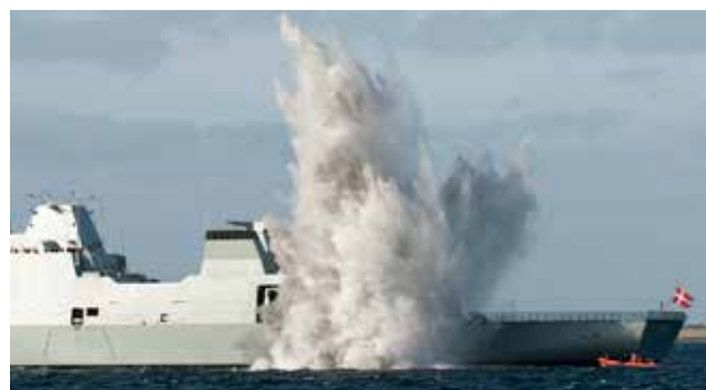
Full-scale shock testing – from underwater explosion
