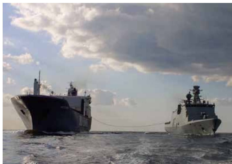
Preparing replenishment at sea (RAS operation) while under way
