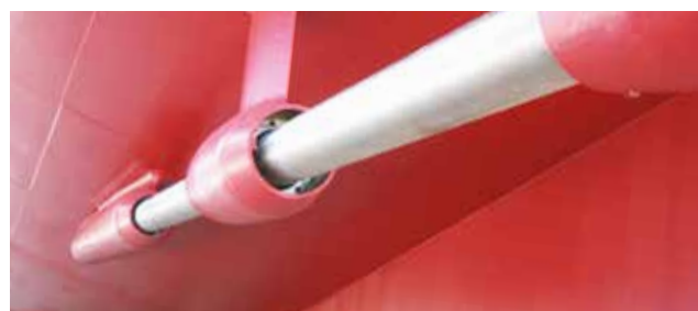
Shafting: Struts, bearings and a clad-welded tail shaft
