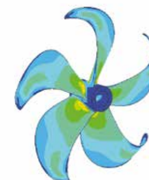
Blade roots Von Mises stresses in wake field, normal loading
