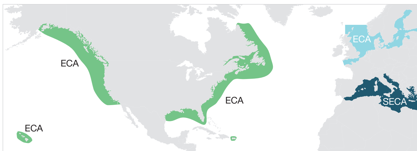
Fig. 4.05: Existing SO x & NO x emission control areas around North America and North Europe, and SO x emission control area in the Mediterranean
