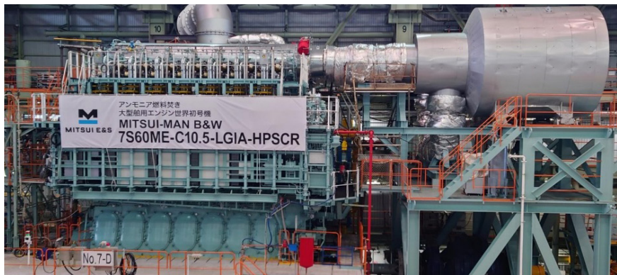
Fig. 7: 7S60ME-LGIA engine at Mitsui
