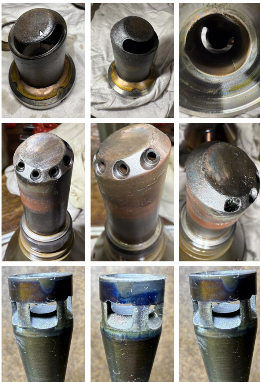
Fig. 27: First inspection of mini-sac fuel valves after 683 running hours on diesel fuel shows that the nozzle and cut-off shaft are in good condition
