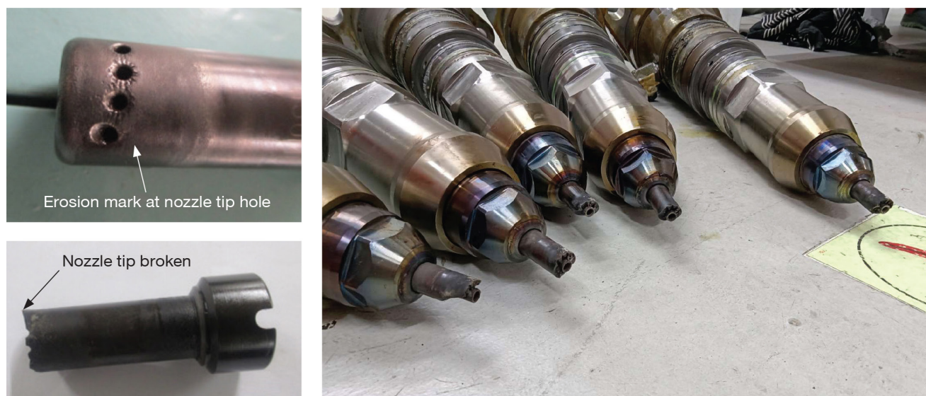
Fig. 2: During Tier III operation, fatigue damage occurred on injector nozzles from a G50-LGIM-W engine
