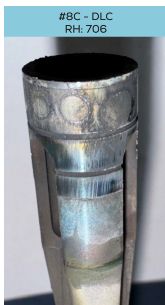
Fig. 28: Erosion on the tip of the cut-off shaft from the slide-version of the methanol fuel valve for G95 LGIM
