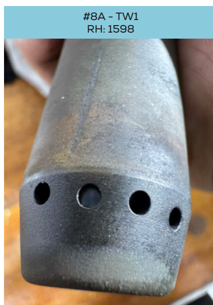
Fig. 28: Erosion on the tip of the cut-off shaft from the slide-version of the methanol fuel valve for G95 LGIM
