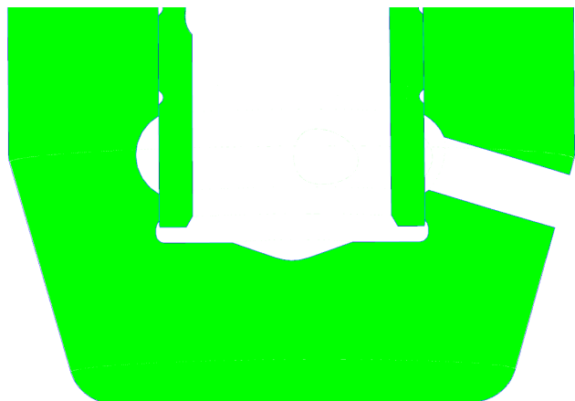
Fig. 30: Methanol slide-type nozzle with standard sealing length: a) 0.8 mm and b) Test design with increased sealing length: 1.2 mm
