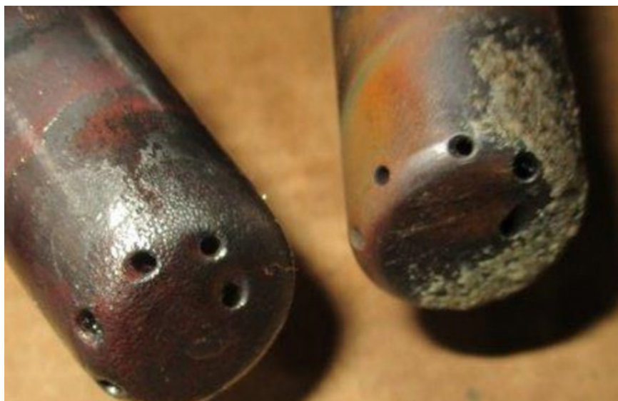
Fig. 22: Inconel nozzles, which have completed over 5,000 running hours in LGIP engine service tests
