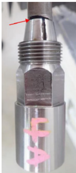
Fig. 3: Original cone design (inner cone indicated by the red arrow)
