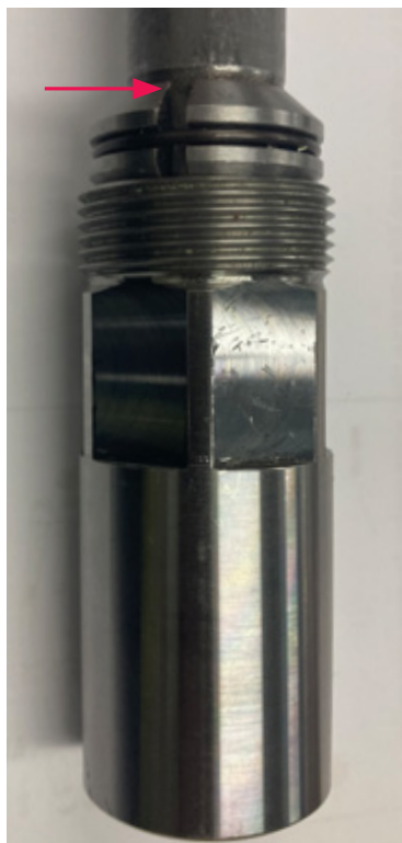
Fig. 4: New 45° cone design (indicated by the red arrow) with a smooth transition to the inner pipe and b) stress simulation of the new cone design
