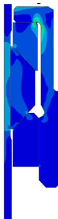
Fig. 4: New 45° cone design (indicated by the red arrow) with a smooth transition to the inner pipe and b) stress simulation of the new cone design
