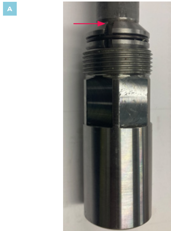
Fig. 4: New 45° cone design (indicated by the red arrow) with a smooth transition to the inner pipe and b) stress simulation of the new cone design
