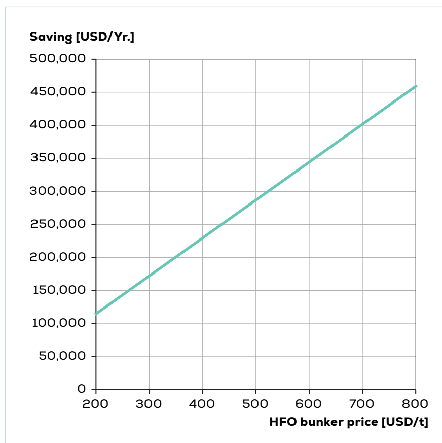
Fig. 25: OPEX saving as a function of HFO bunker price
