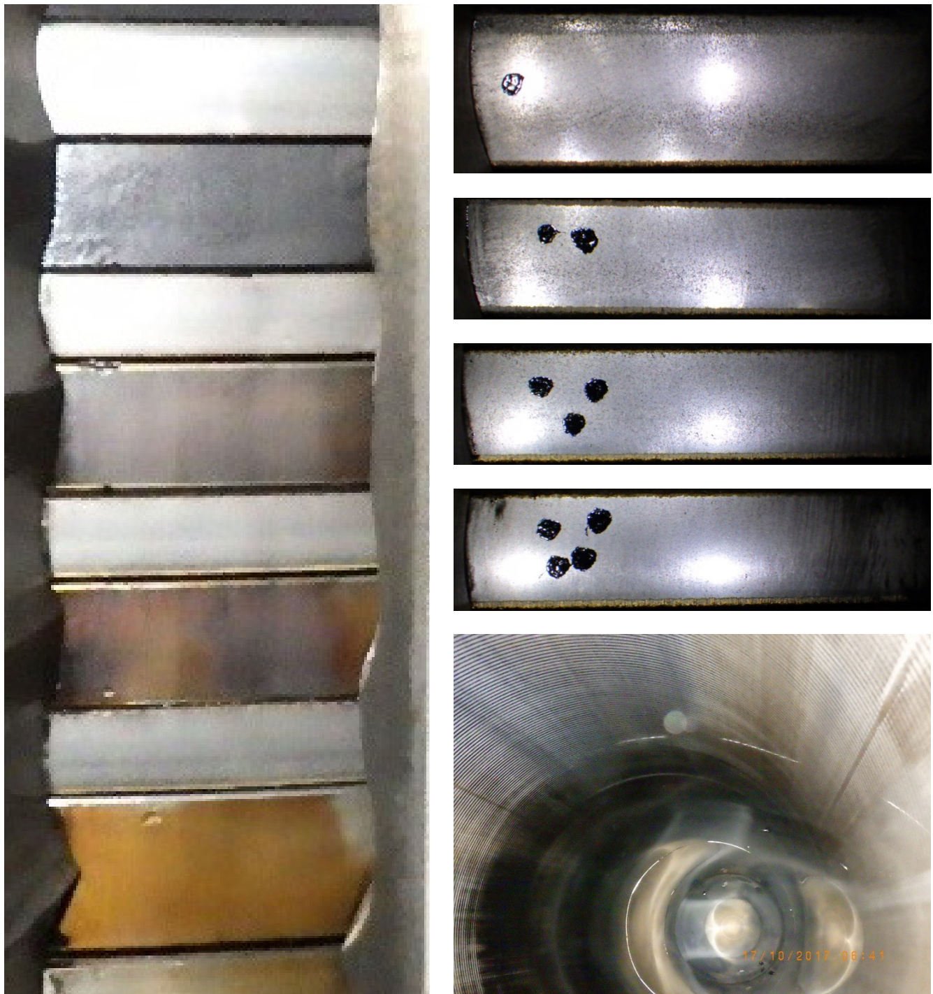
Fig. 24: Ring pack and combustion chamber with visible wave-cut after 7,058 running hours on methanol
