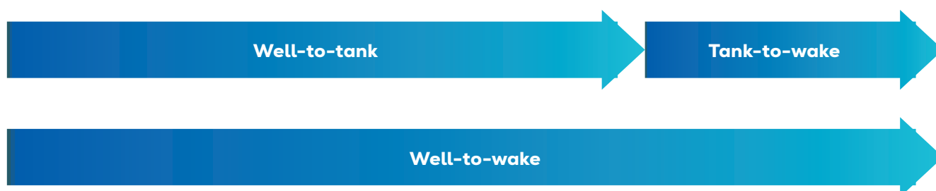
Fig. 9: Emission scopes: tank-to-wake, considering on-board emissions, well-to-wake, considering upstream emissions from the production of the fuel as well
