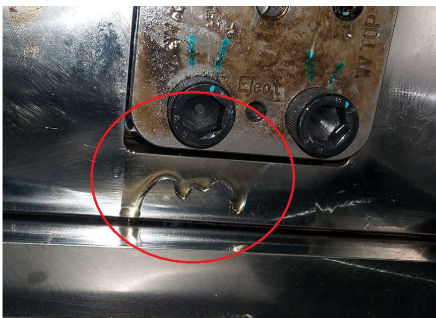
Fig. 21: External sealing oil leakage from the window valve
