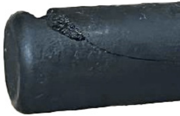
Fig. 28: Original compound type PIV nozzle with cracks
