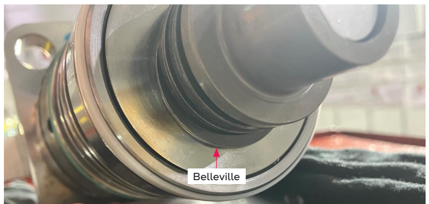
Fig. 15: The spring cup was introduced in a revision of the design
