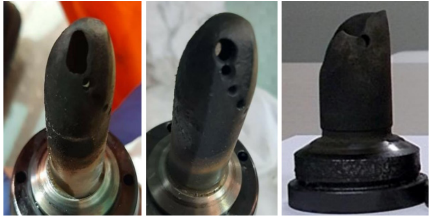
Fig. 24: Long nozzle design with heavy hot corrosion
