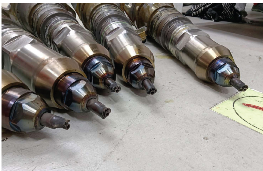
Fig. 2: During Tier III operation, fatigue damage occurred on injector nozzles from a G50-LGIM-W engine
