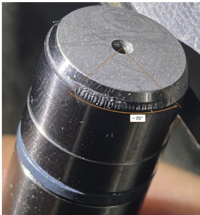
Fig. 22: Erosion damage of blow-off valve spindle for G95ME-C10.5-LGIM
