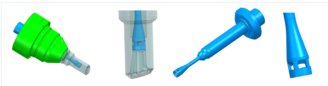
Fig. 26: Details of the mini-sac design
