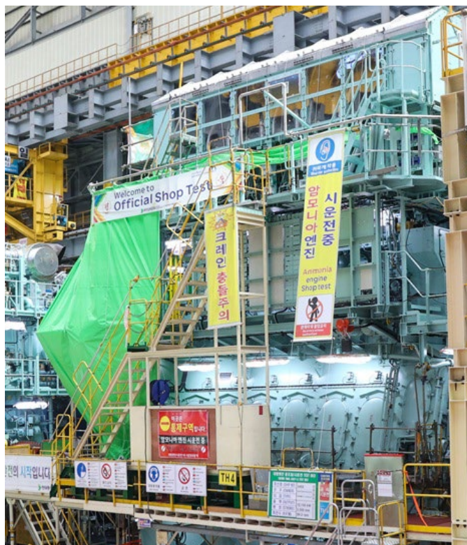
The Everllence B&W 6G60ME-LGIA HPSCR engine pictured at Engine & Machinery of Hyundai Heavy Industries during its Factory Approval Test
