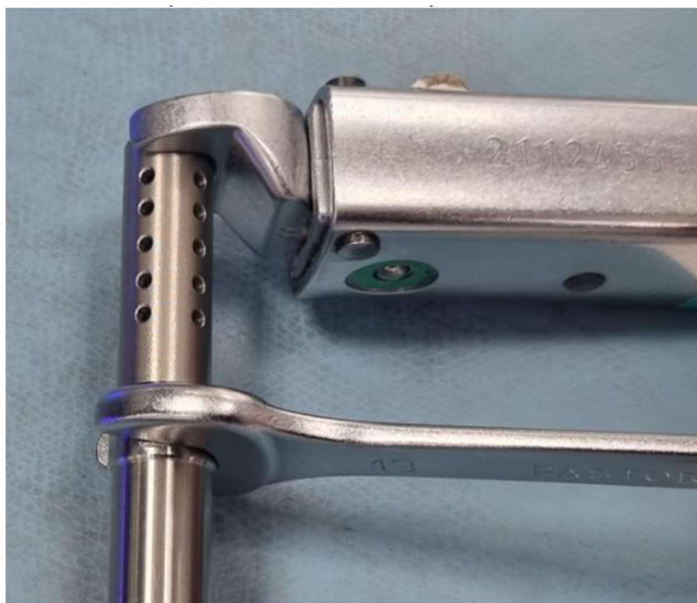
Figure 2. To tighten the filter to recommended 5 Nm torque, please use suitable tool to ensure the torque is correct.
