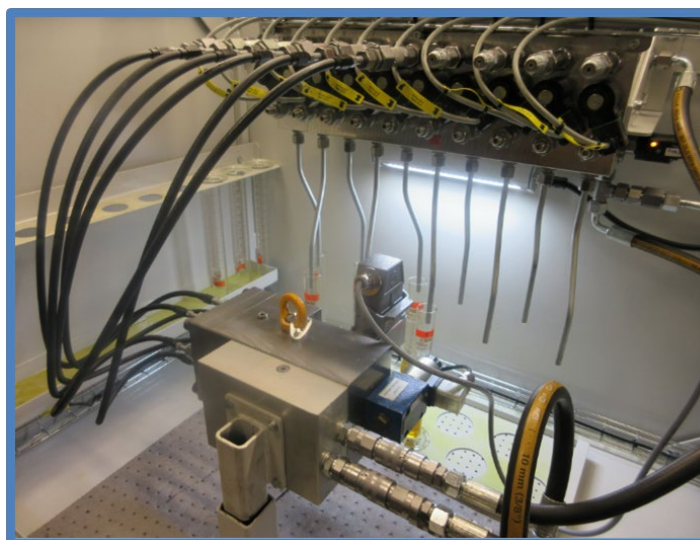
Fig. 2: Alpha lubricator in test rig
