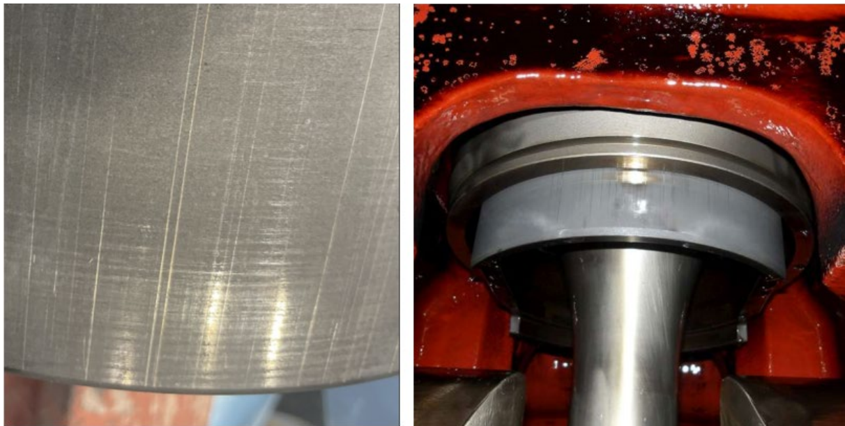
Fig. 1-2: Wear and tear marks on the piston skirt – acceptable for reuse.
