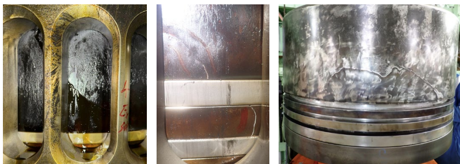
Fig. 1: Example of cracks in piston crowns as observed during scavenge port inspections with the oil pump running and after overhaul and cleaning
