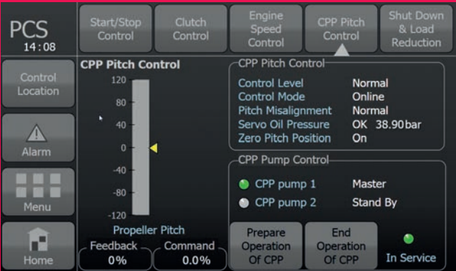
Fig. 18: CPP Pitch Control
