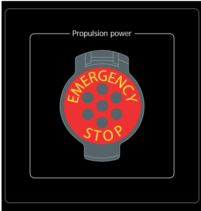
Fig. 24: Emergency Stop Panel – ESP
