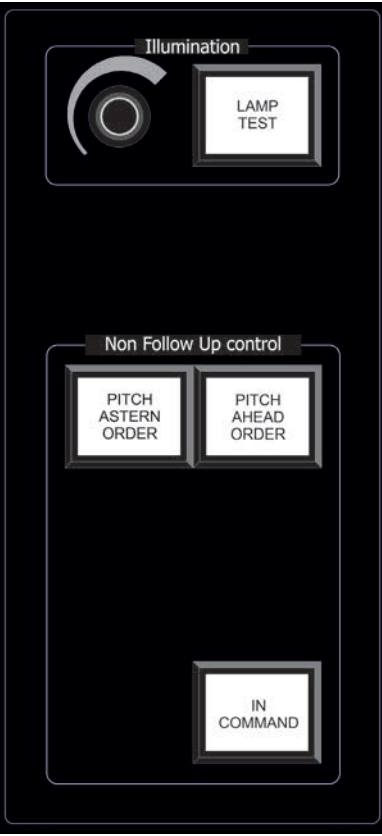
Fig. 26: Non Follow Up control panel – NFU
