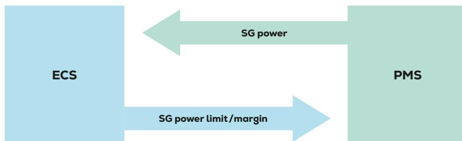
The ECS sends information to the PMS about the power margin to engine overload, thereby enabling the PMS to adjust the PTO load and avoid engine overload. The PMS returns information about the current PTO load to the ECS.
