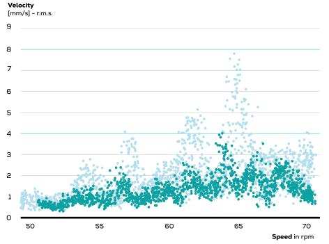
Navigation deck – longitudinal vibration Overall frequency-weighted r.m.s. velocity (mm/s)
