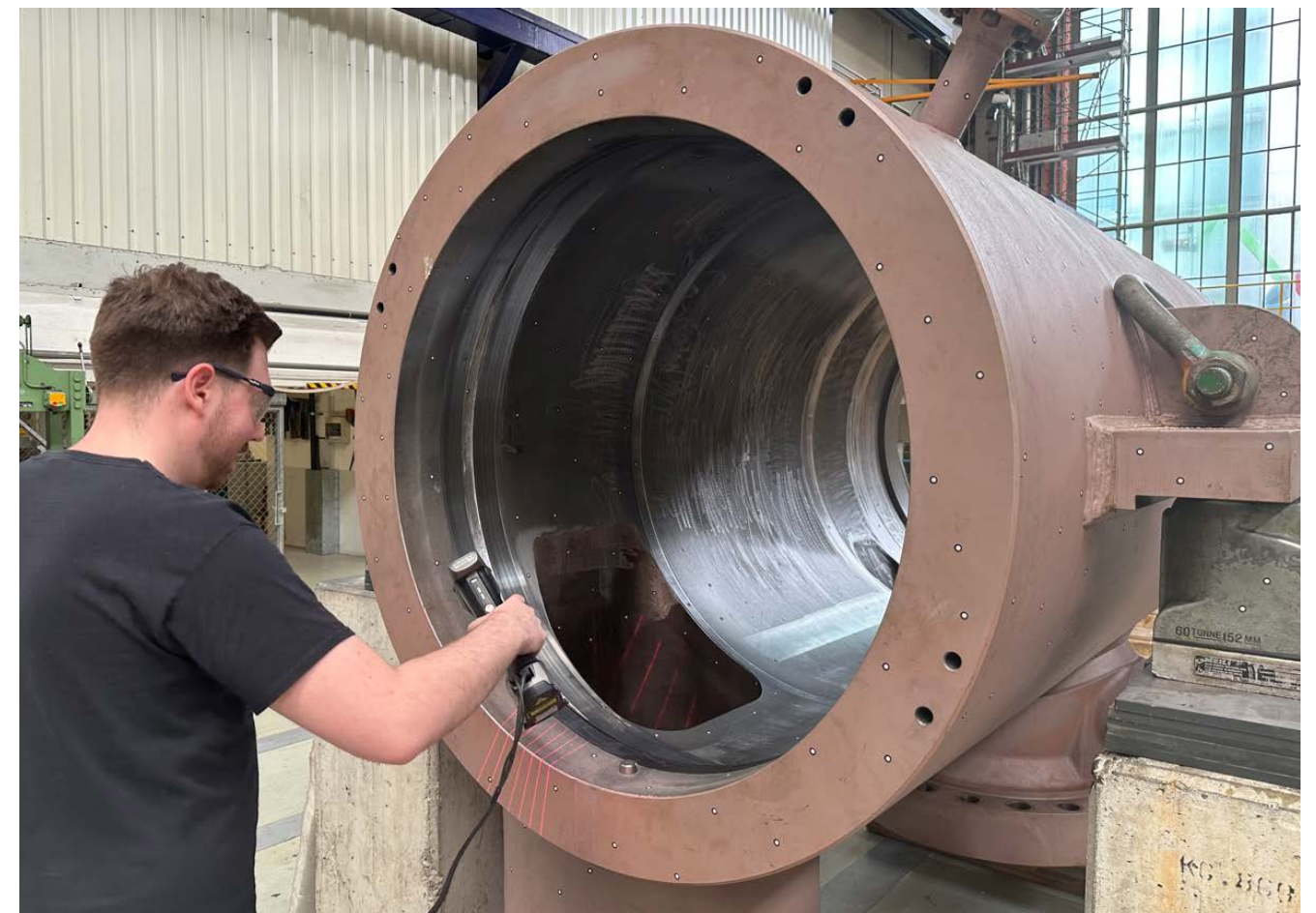
Fig. 2: 3D scan of a barrel compressor outer casing
