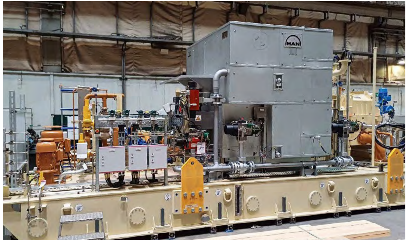
CO 2 turbine skid for Energy Dome
