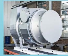
For appropriate tests with the new turbocharger and a 32/40CD, such an engine was initially borrowed from a licensee and imported into the EU. The engine was then subjected to various extensive tests on an engine test bench at our site in Augsburg together with a prototype of the TCF turbocharger, and the high potential fuel savings were confirmed.
